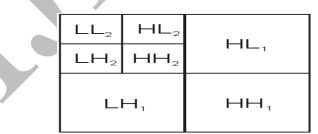
Figure 1: Two Scale 2-Dimensional Discrete Wavelet Transform
