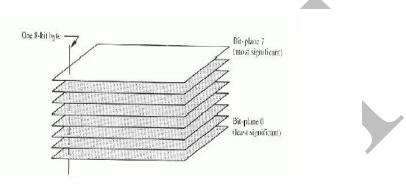
Figure 2: Bit-plane representation of an 8-bit digital image.
